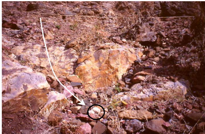
Fig. 5. Tracers (white limestone) displaced over a distance of 6 m in 20 months (Harena rangeland, March 2001). The horizontal rope at the back witnesses original tracer position.
