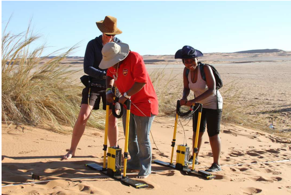
Figure 4: IAG sponsored students Nandipha Mabuza, Christel Hansen and Johanna Niipele using the Ground Penetrating Radar to image the internal structure of the dune (G. Wiggs)
