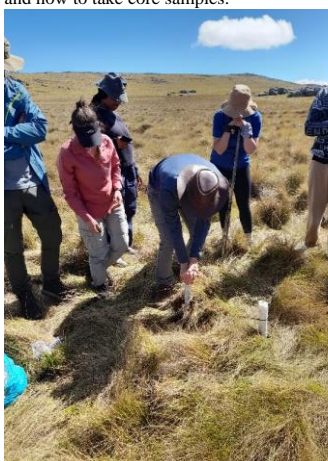
Jason Le Roux explaining the peat auger and how to take core samples.
