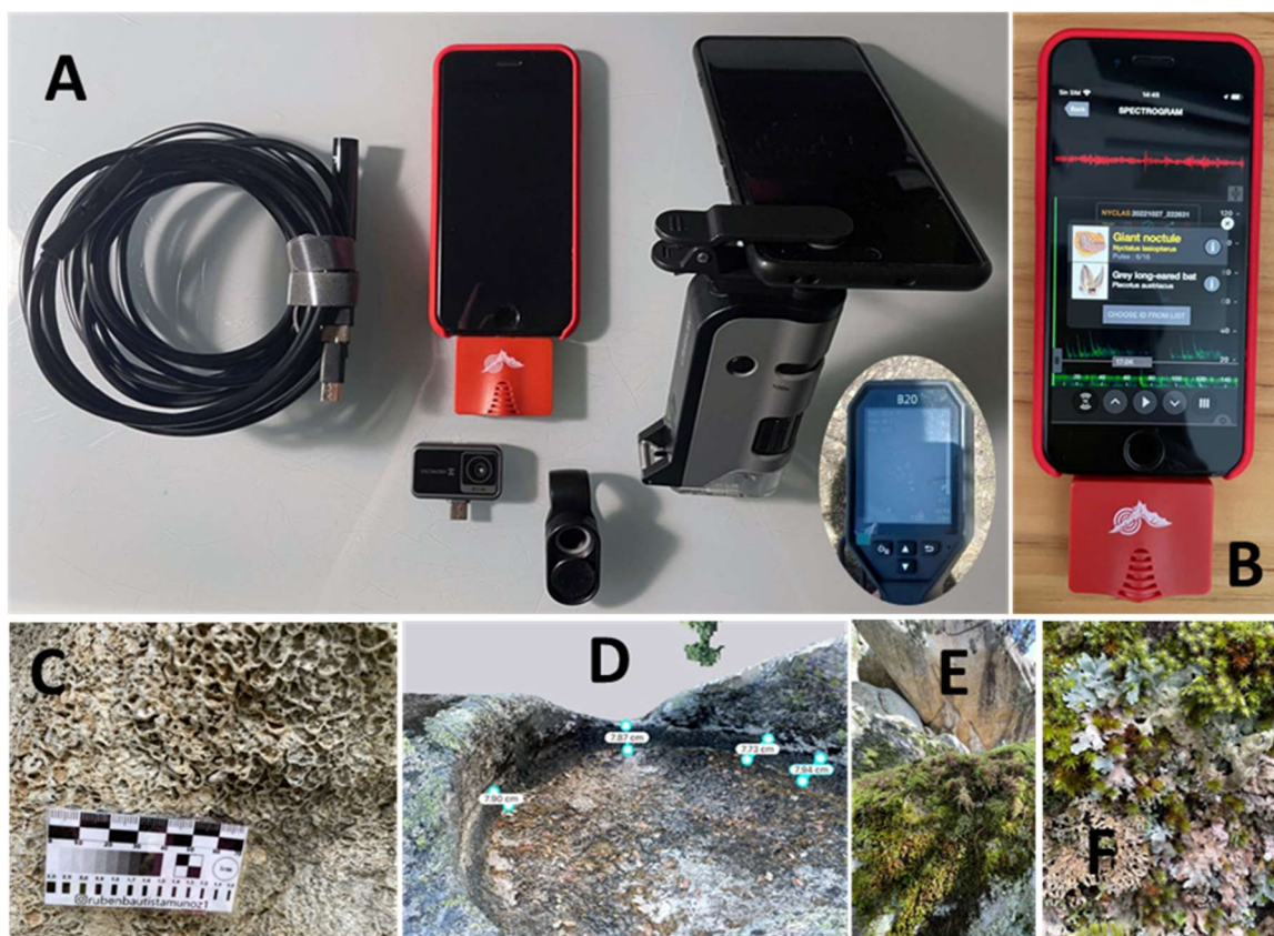
Figure 1. A. Equipment used for digitization in the work: endoscopic camera, Hikmicro thermal camera for mobile phone (accuracy 0.05° C); Echometer Touch 2 ultrasound detector for surveying bats; mobile microscopes 250X, handheld thermal camera. B. Greater noctule detected in La Pedriza. C. Siliceous speleothems microgour in La Pedriza. D. 3D model obtained with an iPhone 12 Pro. E. Hypnum cupressiforme and Hedwigia in La Pedriza. F. Cladonia and beneath Sytrichias.
