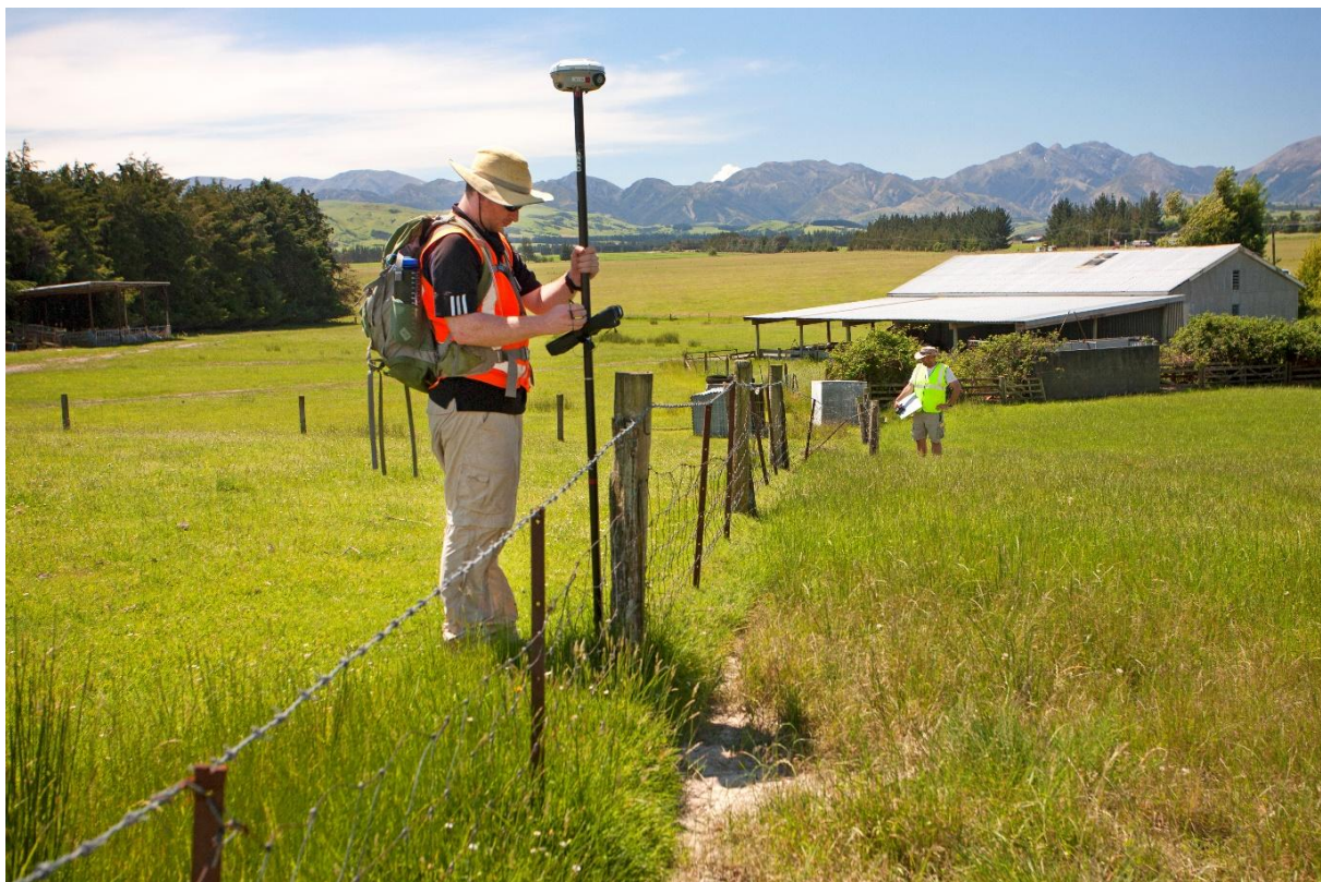
Figure 7. Photograph (looking north) of displaced fence on The Humps Fault, Dalmer Property, near Waiau (Photograph Kate Pedley).
