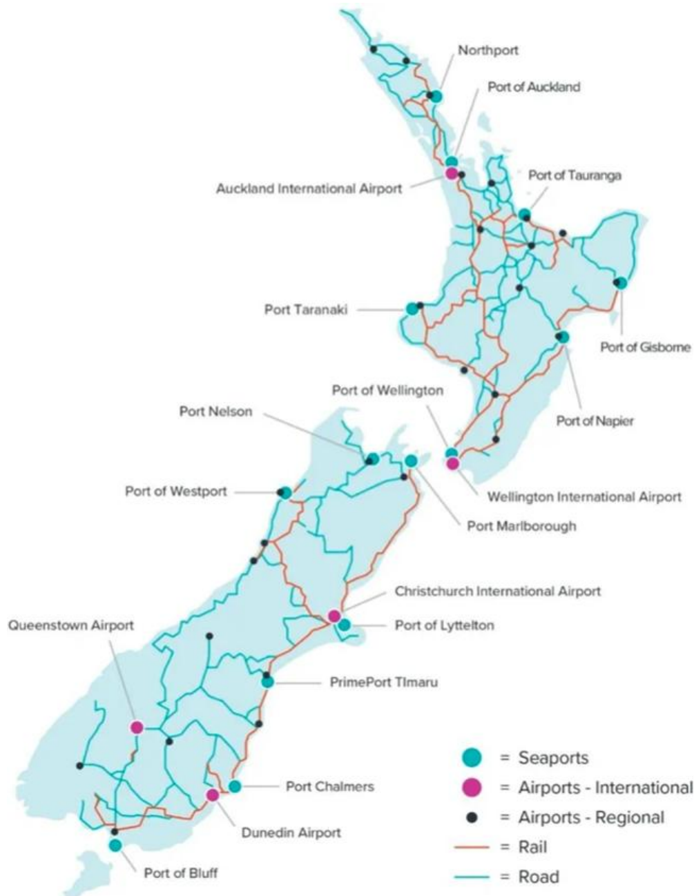
Figure 3: Critical transport infrastructure across New Zealand. The lack of redundancy in routes across the Southern Alps makes the road and rail links through Arthur's Pass critical pinch points.
