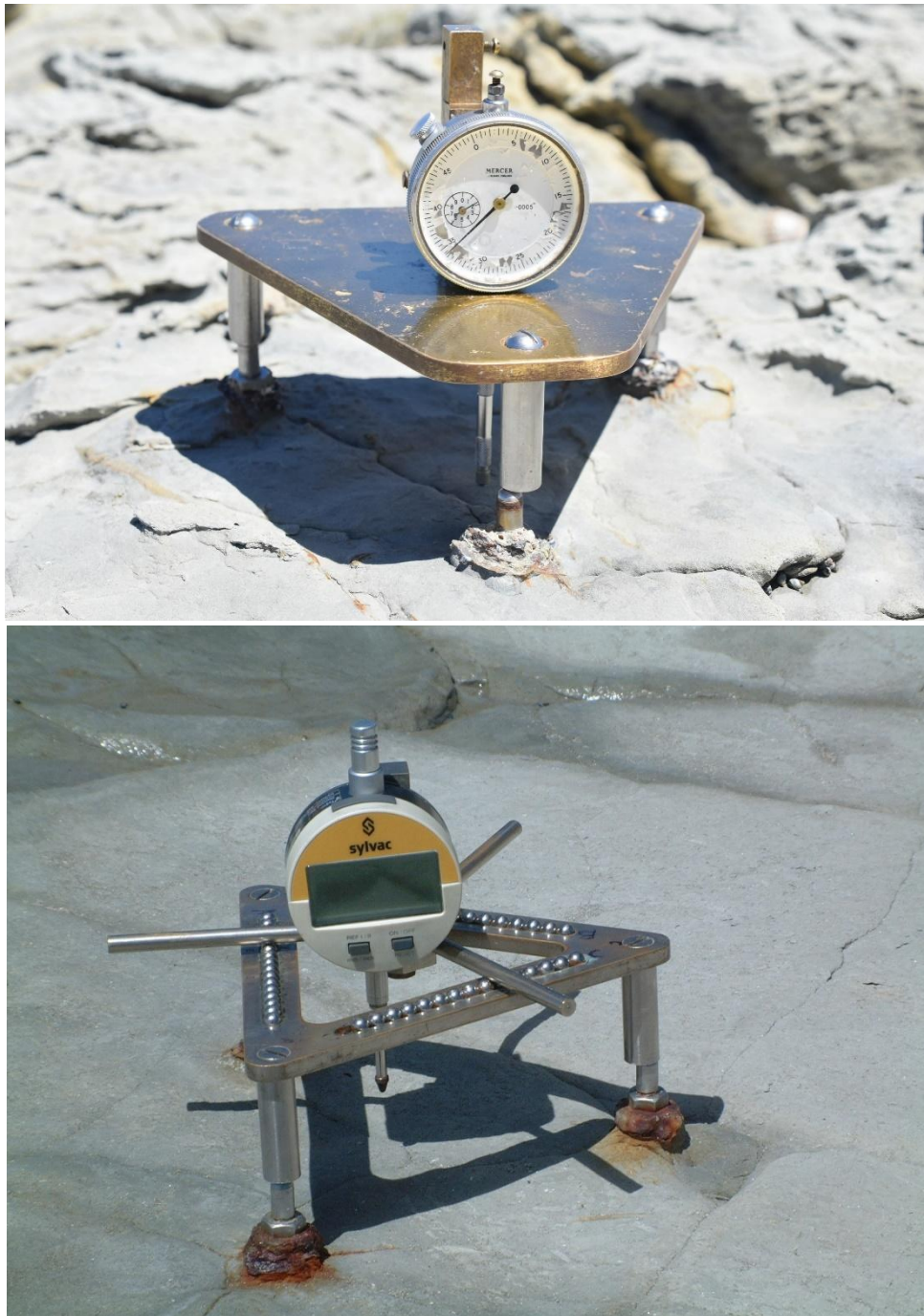
Figure 7. Micro-erosion meter (a) meter used at Kaikōura since 1973 that records 3 measurements and b) the traversing Micro-erosion meter used since 1993 that records 120 measurements.
